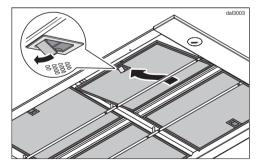
■ To take out a grease filter, release the locking clip on the filter, lower the filter slightly, unhook it at the back and remove it.
